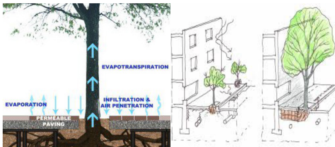
Typical soil cell section showing air intrusion Typical soil volume vs soil cell section
