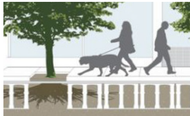
Typical travel zone soil cell section
