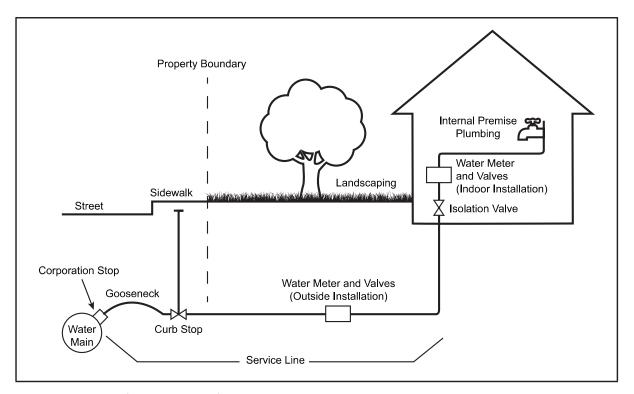
Figure 1 Typical water service line components
