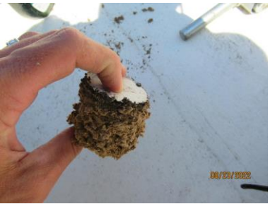
METAL DECK 1.5" PERLITE MOD BIT COATING
